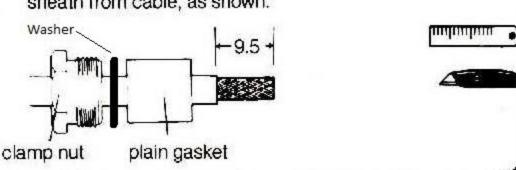
Pold back braid and push ferrule over dielectric to trap braid between outer sheath and ferrule. Trim off surplus braid.
